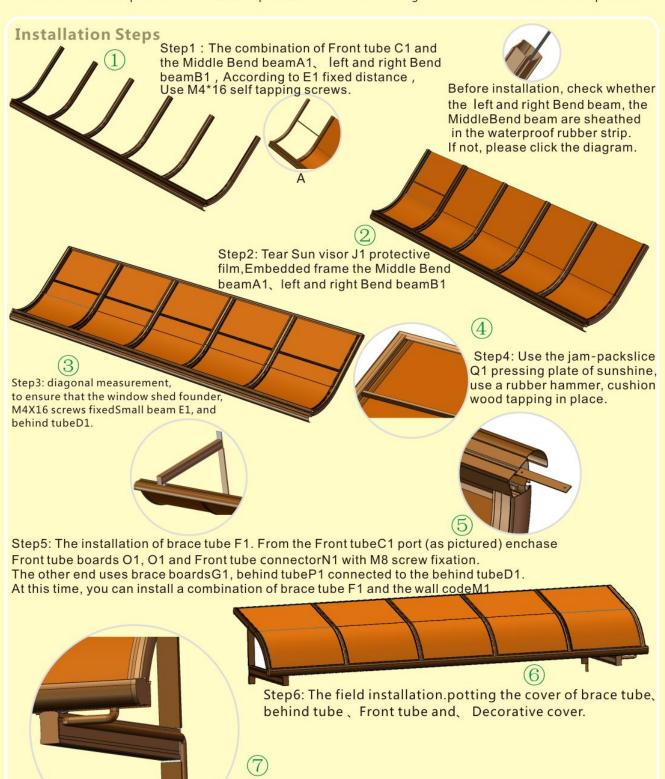
Step7: Installation of drainage system. The use of M4\*30 screw fixed, then ABST1, Pipe connectorR1, ElbowS1, sewer pipeH1&H2 connection.
