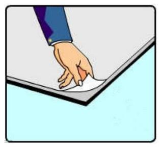
Bighands Polycarbonate Solid Sheet's is produced with a protective PE film on both sides which should be kept on until the panel is fastened. The UV protected side is to be faced towards the sun and is marked with printed film.
