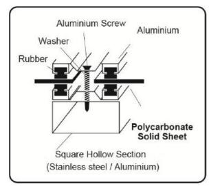
Make sure the support structure is clean and dry. Do not directly screw the sheet, only use aluminium clapping for joining. Must leave a gap of at least 5mm in between sheets for thermal expansion and contraction. A minimum slope of 5° roof pitch is recommended to allow adequate rain water run-off.
